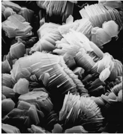
Figure 6.2 Electron micrograph of kaolinite clay minerals magnified 4700 \times . Note the platy or flaky appearance of the pseudo-hexagonal kaolinite crystals, which are arranged in this specimen in distinct “books.”
