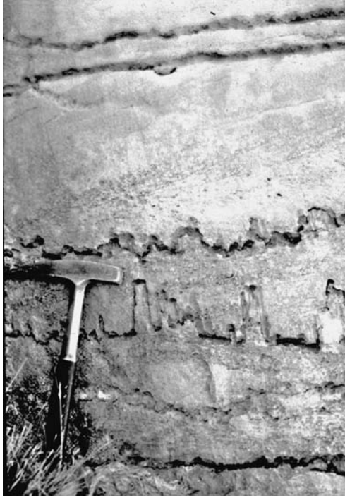
Figure 11.9 Well-developed, sutured stylolites in limestone. Cretaceous limestone, Calcare Massiccio, Italy. (Photograph courtesy of E. F. McBride.)
