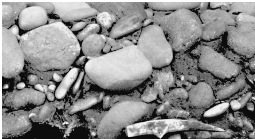
Figure 5.2 Clast-supported fabric in terrace gravels of the Umpqua River, southwest Oregon. Clasts are in contact and thus form a supporting framework. Hammer head for scale.
